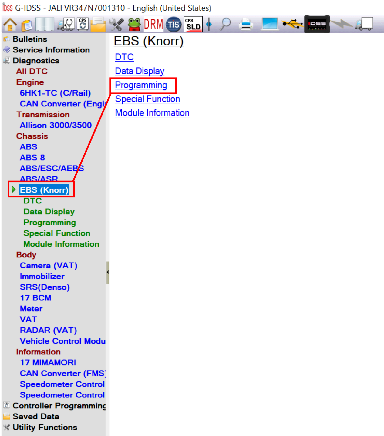
Figure 3 Select EBS (Knorr) from the Diagnostic Menu, then Select Programming.
